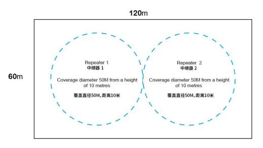
Each blue circle shows the coverage area from a repeaterunit mounted on a roof beam 10M high
